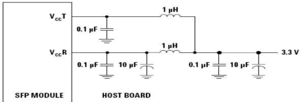
Note: Inductors with DC resistance of less than 1Ω should be used in order to maintain the required voltage at the SFP input pin with 3.3V supply voltage. When the recommended supply filtering network is used, hot plugging of the SFP transceiver module will result in an inrush current of no more than 30mA greater than the steady state value
