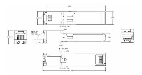
Figure 2. OLSTMRR-CNS1 mechanical dimensions
