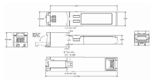
Figure 2. TOP-SFP-TF2 mechanical dimensions
