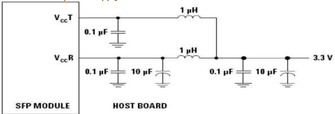
Note: Inductors with DC resistance of less than 1Ω should be used in order to maintain the required voltage at the SFP input pin with 3.3V supply voltage. When the recommended supply filtering network is used, hot plugging of the SFP transceiver module will result in an inrush current of no more than 30mA greater than the steady state value
