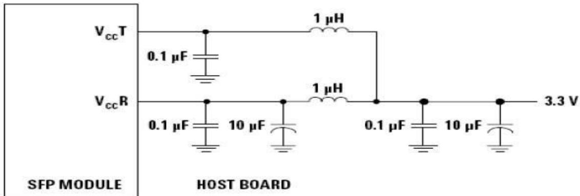
Note: Inductors with DC resistance of less than  $1\Omega$  should be used in order to maintain the required voltage at the SFP input pin with  $3.3\text{V}$  supply voltage. When the recommended supply filtering network is used, hot plugging of the SFP transceiver module will result in an inrush current of no more than  $30\text{mA}$  greater than the steady state value.
